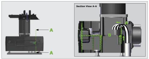
FIGURE 42. CABLE ROUTING FOR NEW INSTALLATIONS
