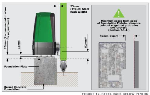
Includes 3mm clearance required between Rack and Pinion
