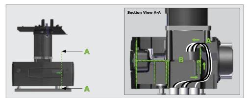
FIGURE 43. CABLE ROUTING FOR RETRO-FITS WITH LONGER CABLES
