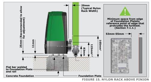
Includes 3mm clearance required between Rack and Pinion
