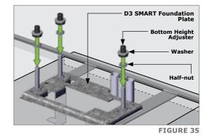
Adjust the Half-nuts to be 12mm clear from the Foundation Plate.
