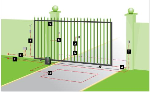
**FIGURE 7. CABLING REQUIREMENTS**
