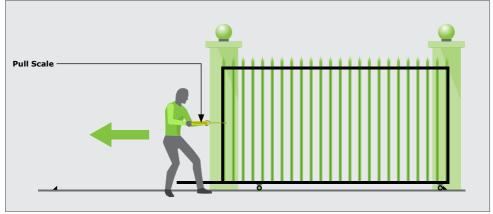
FIGURE 6. STARTING AND RUNNING FORCES
