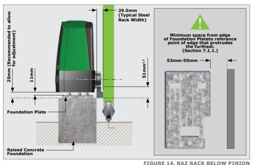
Includes 3mm clearance required between Rack and Pinion
