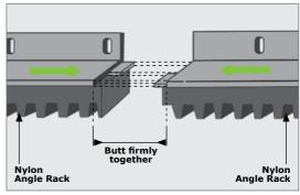
When joining two lengths together, simply butt each section firmly together to ensure that the correct pitch is achieved.
